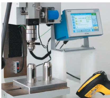
The KVC 821 optical inspection system from Kistler provides automated quality assurance at the end of the production line
