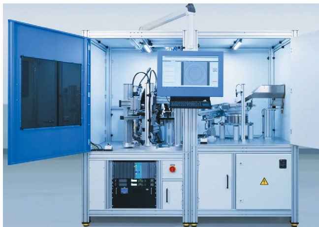
Seven test automation systems of the new generation KVC 821 from Kistler form an integral part of Zinktechnik's highly automated zero-defect production of zinc casting parts in high volumes
