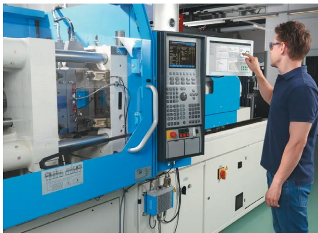
ComoNeo from Kistler is the leading process monitoring system to ensure high quality and transparency in injection molding production
